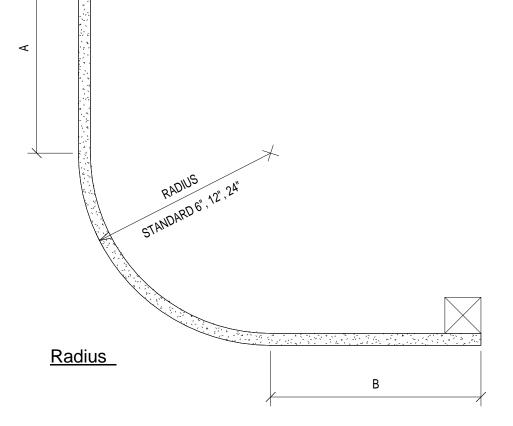
TO USE REVIT FAMILY: -INSERT COMPONENT INTO PROJECT -PLACE COMPONENT USING 'PLACE ON FACE' OR 'PLACE ON WORK PLANE' DEPENDING ON ORIENTATION REQUIRED. -CREATE TYPES AS REQUIRED TO SUIT PROJECT, FOLLOWING THE PARAMETERS BUILT INTO EACH FAMILY. -TOGGLE DETAIL LEVELS TO VIEW DETAIL COMPONENTS. -FAMILY MATERIAL IS "GYPSUM WALL BOARD - CURVED WALLS"
